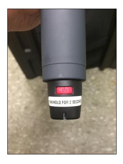
To turn on the Microphone press and hold the red button for 2 seconds. When not in use it's a good idea to turn off the Microphone to save the batteries.
