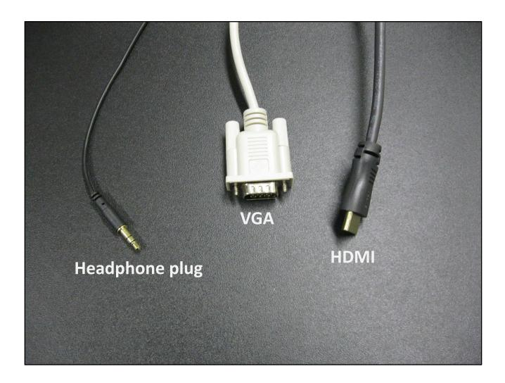
**HDMI** can be used for laptops with HDMI output, as well as iPads and iPhones with an adapter (not provided).
